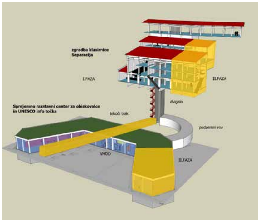
Fig. 4: Drawing of 1st phase of reconstruction of the ore separation plant and construction of the visitors reception and exhibition centre (Rafael Bizjak, 2014); note: yellow section designates area that will not be realised in 1st phase.
