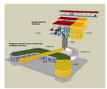
**Fig. 4:** Drawing of 1st phase of reconstruction of the ore separation plant and construction of the visitors reception and exhibition centre (Rafael Bizjak, 2014); note: yellow section designates area that will not be realised in 1st phase.
